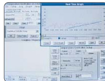
Software features real-time graphing and simple setup of ramp & soak programs
