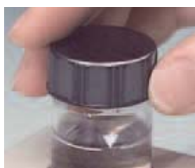
Left middle: Index markings on the cuvettes make it easy to perform repeatable measurements
